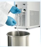
Flexible fill tube on the front panel enables unit to be drained quickly.
